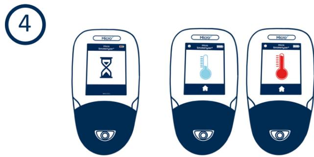
4 Allow the Micro+™ monitor to zero. If the monitor is too cold or hot please wait for it to come to ambient temperature before continuing
