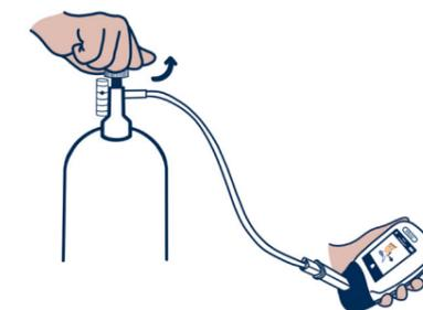
Once the countdown has finished and the screen prompts to exhale, open the gas regulator to perform the bump test
