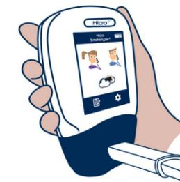
As routine maintenance, a bump test should always be performed after long periods of no use to check the device is reading correctly. You can perform a bump test using either a non-smoker or certified gas to ensure the device is reading correctly.
