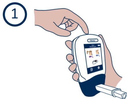
1 To perform a calibration test, firstly turn on the Micro+™ monitor
